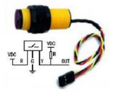
Figure 4. Infrared sensor E18-D80NK.
