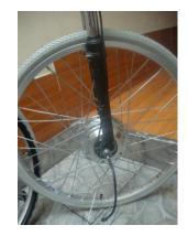
Figure 8. Brushless motor coupled to the wheelchair rim.
