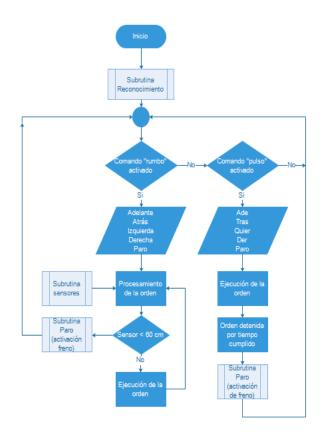
Figure 11. Basic system flowchart
