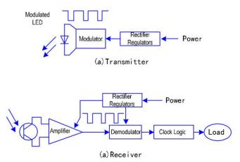
Figure 5. Infrared sensor operation.
