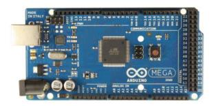
Figure 6. Arduino Mega 2560
