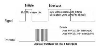
Figure 3. Ultrasonic sensor operation.
