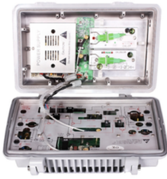
Fig. 21 Optical node in an HFC network.
