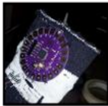
Figure 7.- Arduino Lilypad sewn completely to the wristband (Prototype#2) Source: Edison Flowers
