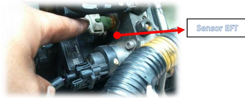
Figura 43. Sensor EFT
