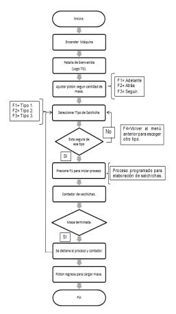
Figure 4.1. Schematic flow chart control. Source. Author
