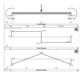
Figure 3.7. shear , bending moment ( Mdsolid) Source. Author.
