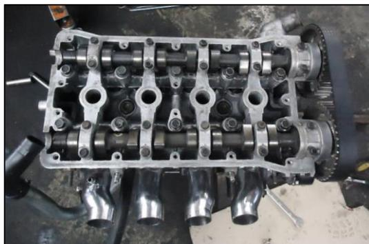
Figura 59. Culata Aveo DOHC (Dual overhead camshaft)
