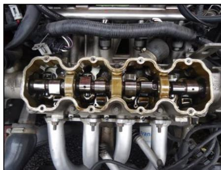
Figura 58. Culata Corsa SOHC (Single overhead camshaft)
