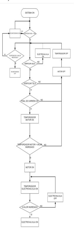
Fig. 3. Flowchart of the humidification and temperature system.
