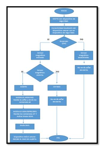
Figure 32. Flowchart of the security system.
