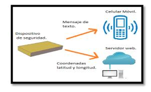
Figure 26. Receiving devices connection.
