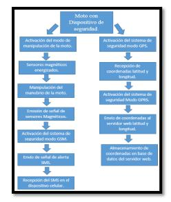
Figure 17. Diagram of operation of the security system.
