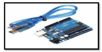
Figure 7. Micro controller ARDUINO.
