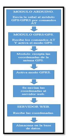
Figure 33. Diagram of operation of GPS and GPRS.
