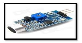
Figure 2. Sound sensor. 3) Sensor for measurement of distance.
