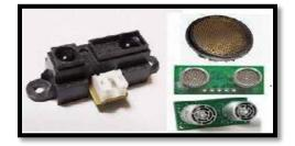
Figure 3. Sensor in measurement of distance.
