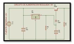
Figure 28. Regulated power supply circuit.
