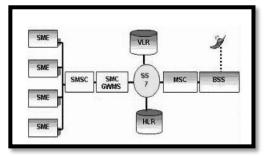
Figure 10. SMS network architecture.
