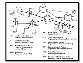
Figure 9. Architecture GSM.
