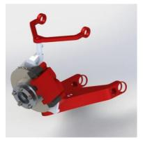
Figure. 6. Front suspension.
