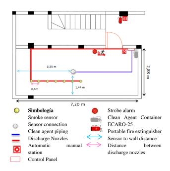
Figure 19. Schematic of the fire detection system Source: Author
