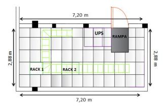
Figure 16. Ladder Location for Electrical Wiring Source: Author
