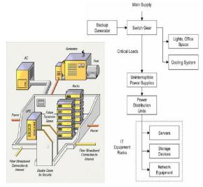
Figure 2. Electrical System Connections Source: POWER HOST. Obtained from: Conectividad y estructura de red. http://bit.ly/2eG8Faq
