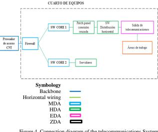
Figure 4. Connection diagram of the telecommunications System Source: Author
