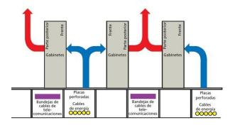
Figure 3. Example of distribution of hot and cold aisles Source: ADC Telecommunications. Obtained from: TIA-942, Data center standards overview, 2005, pag 6
