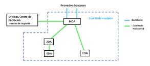
Figure 1. Reduced topology of a Data center Source: ANSI/TIA-942. Obtained from: Telecommunications Infrastructure Standard for Data centers, 2005, pag 25.
