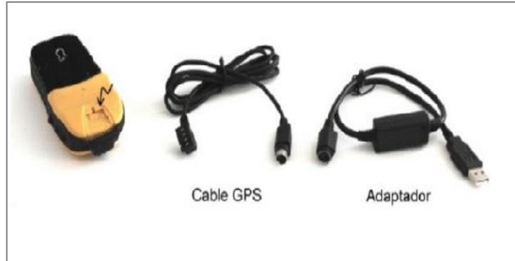
**Figura 5.** Receptor GPS.
