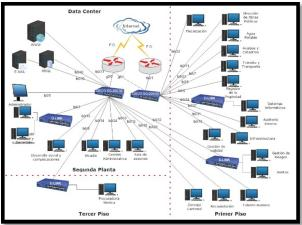
Figure 12. Physical topology diagram
