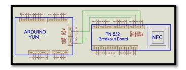
Figura. 5. Connection Plate Arduino Yun and NFC.
