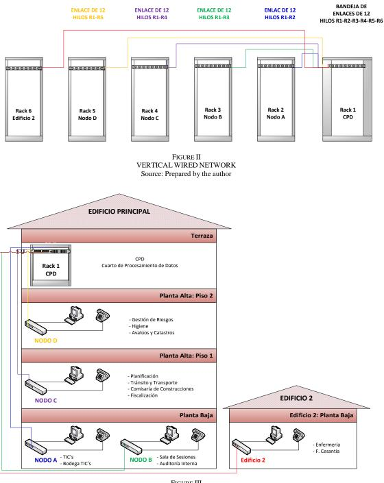
FIGURE III HORIZONTAL CABLING Source: Prepared by the author
