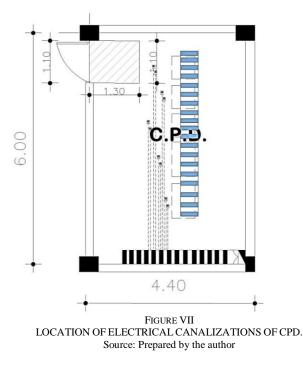
All products of electrical parts are metal (internal and external pipes) taking care of the electrical continuity across the path with their respective identification. These steel or aluminum pipes should not be among them a distance greater than 6<sup>''</sup>. In *Figure VI* the distribution of electrical canalizations is displayed.
