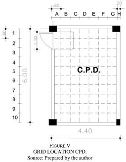
As a rule describes a grid of identifying and locating ICT equipment will be used. In the x-axis (x), they are located uppercase letters A through H; and the ordinate axis (y) have been located numbers from 1st to 10. The dimensions of the grid are of
