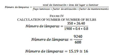
As a result it has the approximate number of 16 lamps. By having two sets of reference 6 each lamp, a system is increased, with a total of 18 fluorescent lamps, distributed as shown in *Figure V*.
