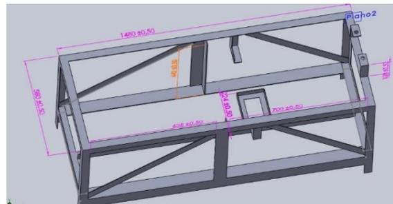
Figure 1: Design Solidwork structure that will support the engine.
