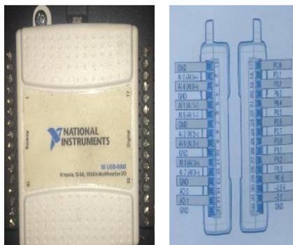
Figure 3: Data Acquisition Board with their pinout
