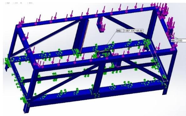
Figure 5: Stress Analysis Static Nodal stress (von Mises).
