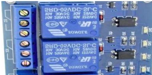
Figure 2: Relay module board.
