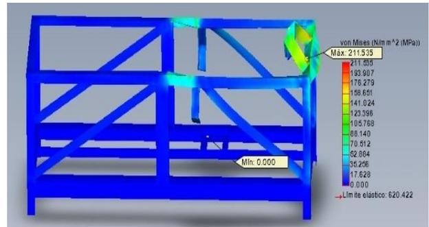
Figure 4: Static Displacement (von Mises)
