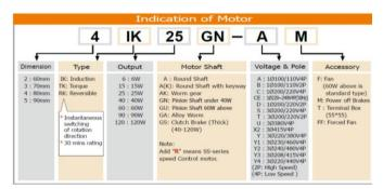
The calculated power is 56.64 W, table engine type 5IK60A-C is selected, this engine has the characteristics of being induction, with a power of 60 W, single phase 220V / 4P, you have to is 1550 rpm, in the figure the observed motor selected.
