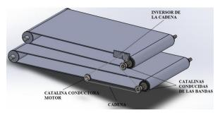
Figure 11: Power Transmission.
