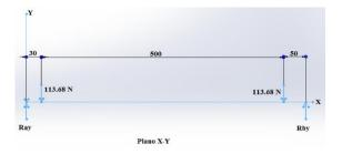
Figure 21: Forces in the X-Y plane.
