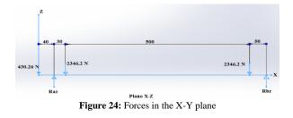
$$\sum_{\substack{R_{az} + R_{bz} - 430.26 \text{ N} - 2346.2 \text{ N} - 2346.2 \text{ N} = 0\\R_{az} + R_{bz} = 5122.66 \text{ N}}}{\sum_{\sum} M_A = 0}$$
