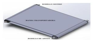
Figure 10: Motor roller and support roller.
