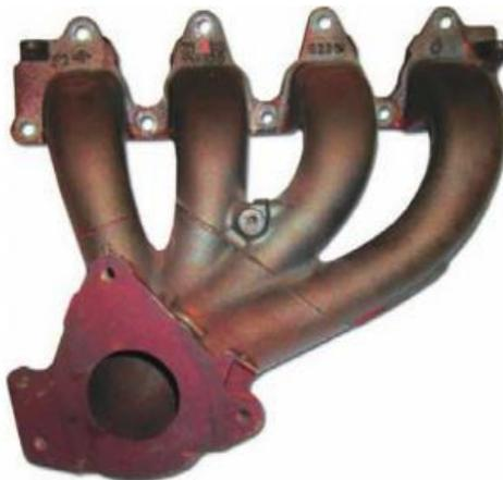
**Figura 1.19** Colector de escape.
